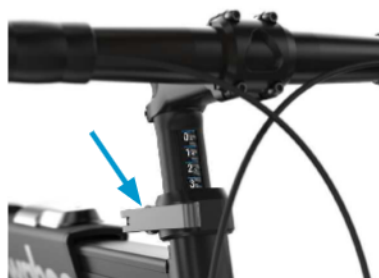
Stack Height Adjustment
