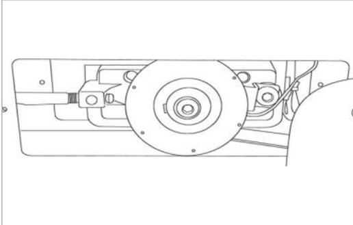
2. Using a long tool, push out the rear end cap as pictured below left. This will give you access to the tank
