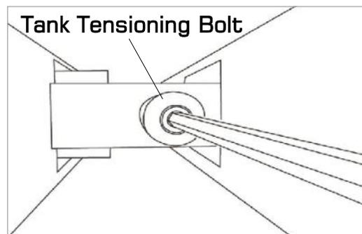
**Note:** Do not over tighten tank Bolts.
