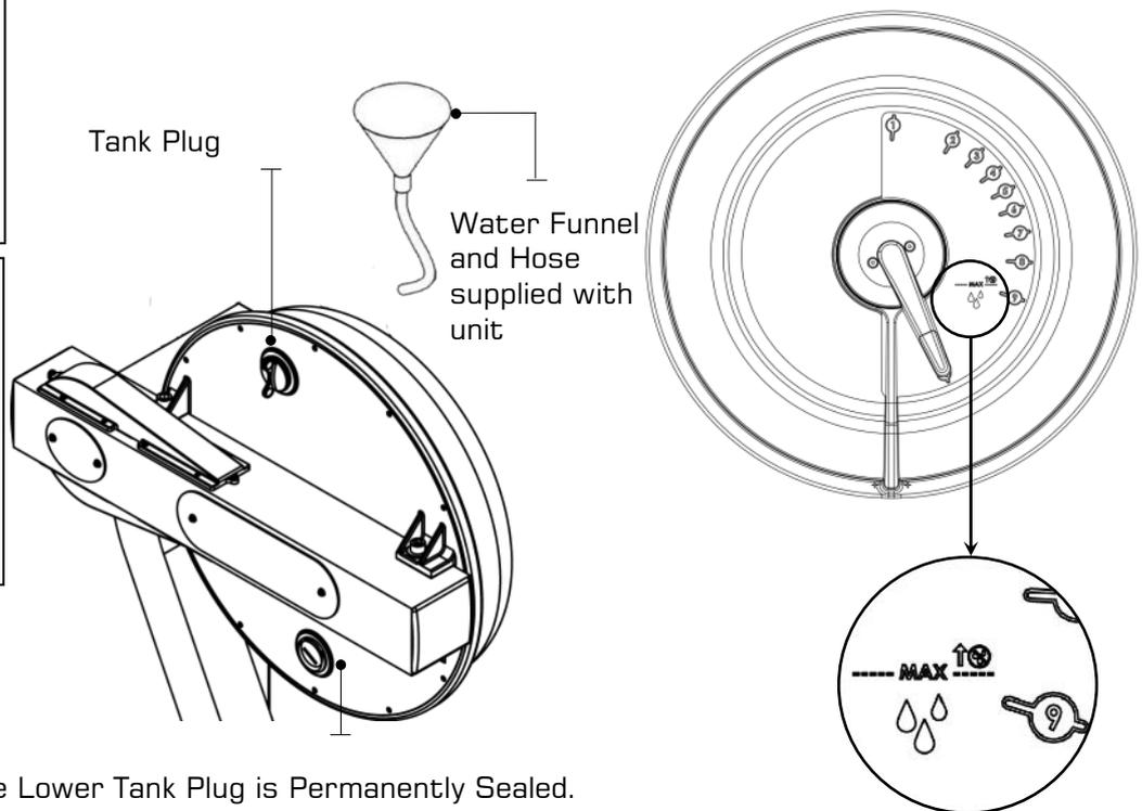
**Note:** The Lower Tank Plug is Permanently Sealed.
