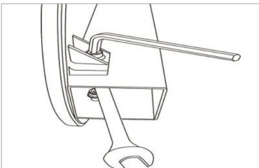
4. Using a 6mm Allen Key, tighten the Belt using the Tank Tensioning Bolt until the belt no longer slips during hard rowing.
