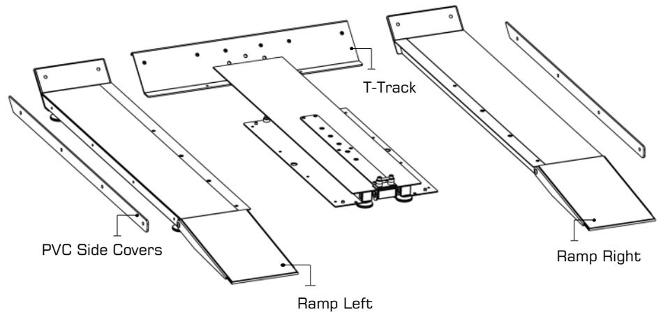
Remove contents from box and make sure all parts are present. Contents will include the T-Track, left/right side Ramps and Bolt pack (note, this may also be located with Seat Assembly).
