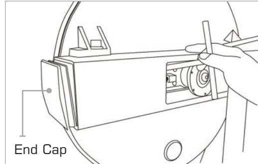
3. Loosen both the rear and front tank Bolts slightly as shown. Remove front Rubber Belt Cover.
